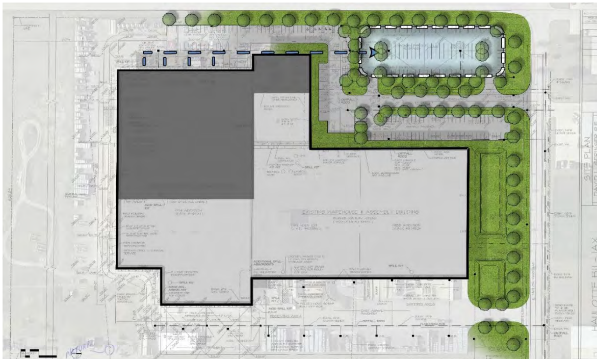
FIGURE 40: UNDERGROUND DETENTION BASIN IMPLEMENTATION EXAMPLE - INDUSTRIAL
