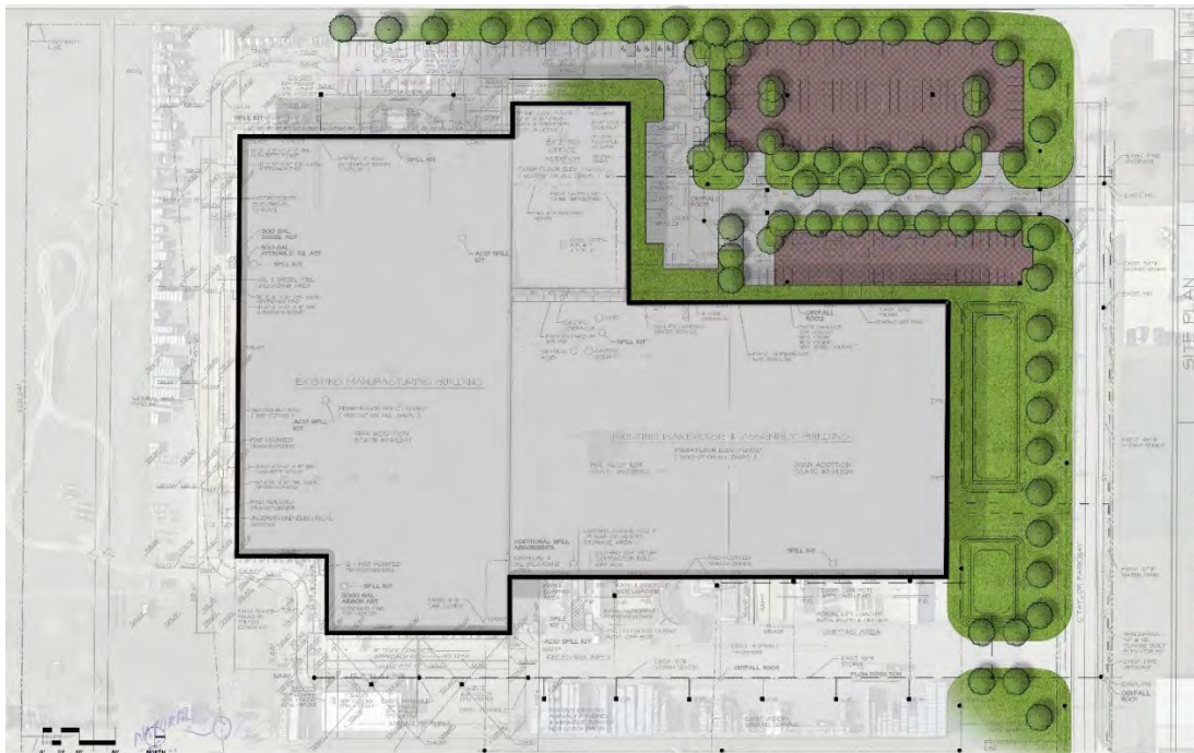
FIGURE 43: PERVIOUS PAVEMENT IMPLEMENTATION EXAMPLE - INDUSTRIAL
