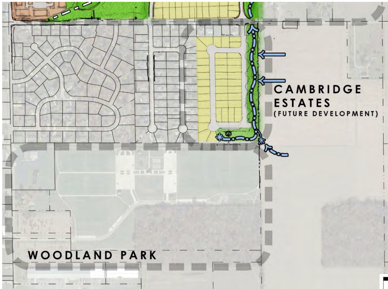
FIGURE 31: BRUSH CREEK CORRIDOR: CAMBRIDGE ESTATES STORMWATER DRAINAGE
